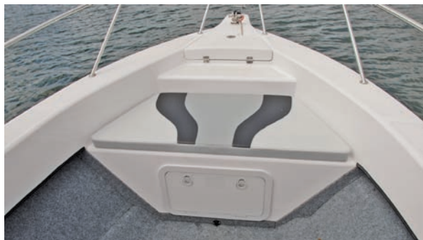
The foredeck treatment allows for easy anchoring and the upholstery can be removed to make the casting platform the place to be in smooth water. There's more storage below.
