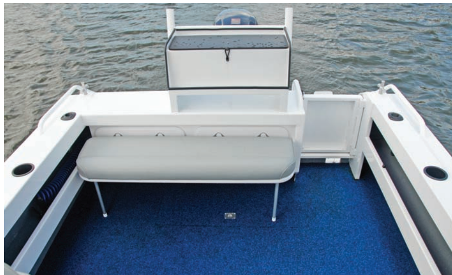
Angling features include side pockets, rod holders, and a rear seat that can fold or be removed if necessary.
