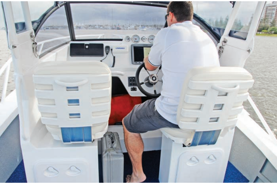
Skipper and mate seats are positioned on top of storage boxes that can be accessed through wide hatches.
