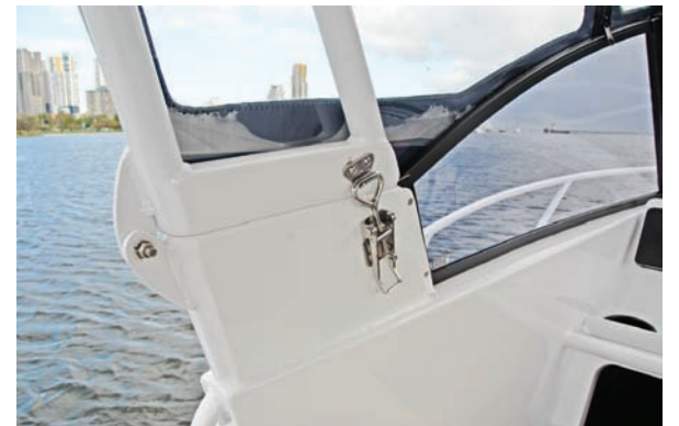
A hinge arrangement on the targa top allows it to fold down out of the way for ease of storage.
